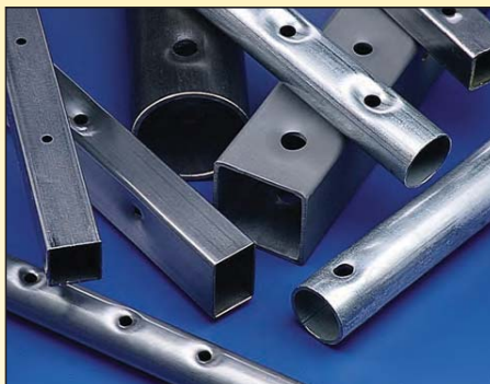
Tube Punching – Round or Square Tubing
